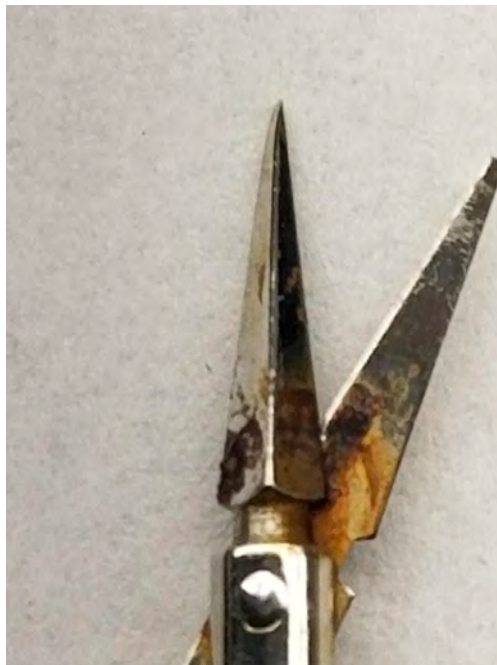
Eye scissor with rust build up
