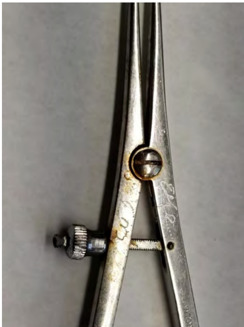
Staining on an eye caliper
