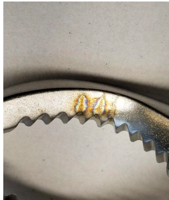
Bone clamp with fractures and staining
