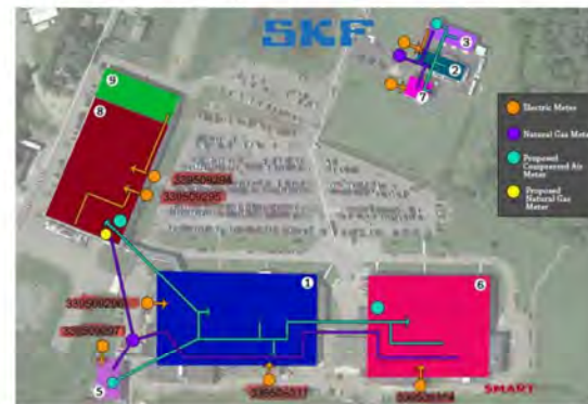
Exhibit 13. SKF Falconer facility map of facility with energy meters marked with their corresponding meter number
